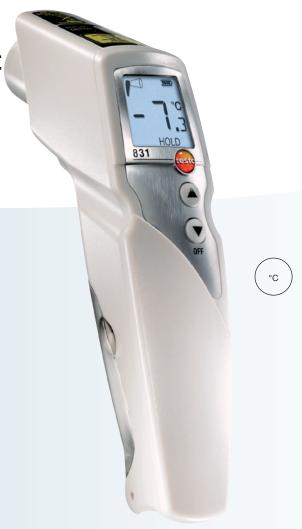
The testo 831 is an infrared thermometer for distance measurement. Thanks to its 30:1 optics, the measurement point diameter is only 3.6 cm at a distance of 1 m.
