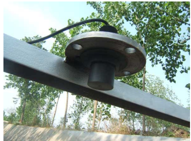
⑧ Finished installation of transducer
