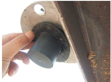
⑧ Finished installation of transducer
