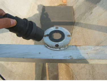
③ Transducer aimed at the hole of flange
