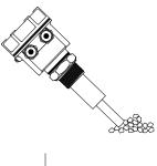
When material touches the rod, vibration stops as resonance gets disturbed.
