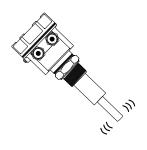
Electronics of LSVR excites the piezo-electriccrystals inside the tuning rod, which makes the rod vibrate at it's natural resonance frequency in free air.
