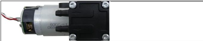
4. Loosen the 4 fastening screws (Torx spanner T 9) on the pump head of the main gas pump.
