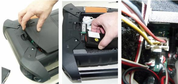
1. Open the cover of the service compartment (locking clip) on the back of the meas. box.
