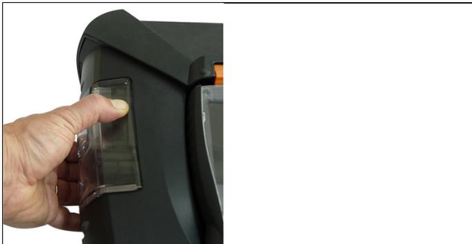
1. Unlock the condensate trap / condensate container by the orange handle on the underside.
