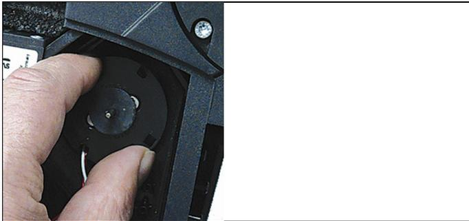
4. Loosen the motor on the condensate pump (short anti-clockwise turn).
