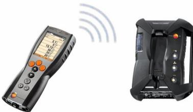
Via Bluetooth® the Control Unit can be connected to a meas. box or a PC/Notebook, as long as both components are equipped with this function, see **Bluetooth®**, page 52.
