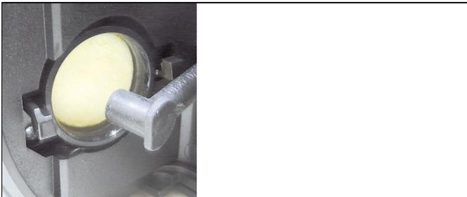
4. Replace the exhausted filter with a new filtration non-woven.
