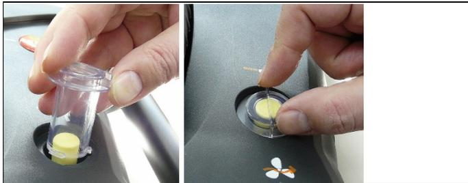
3. Attach the filter cover and lock by turning it clockwise. The rib on the filter cover must be parallel to the handle.
