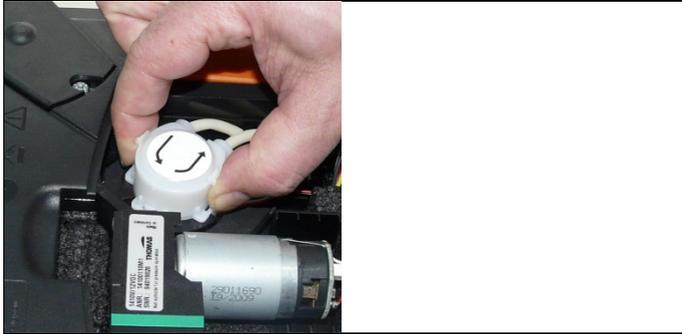
2. Unlock the two lateral clip locks of the condensate pump and pull off the pump head.
