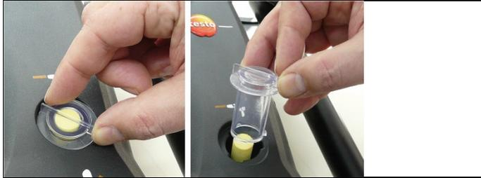
1. Open the filter chamber: Turn the filter cover anti-clockwise and take it off.
