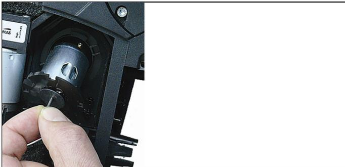
5. Take the motor of the condensate pump out of the bracket.
