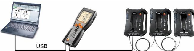
**i** If testo easyEmission software is connected via a control unit to measuring boxes, the number of measuring boxes must not be changed. To add new measuring boxes, end the testo easyEmission software, connect the new measuring box and restart the testo easyEmission software.
