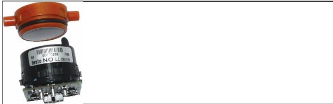
7. Plug the new filter on the sensor.
