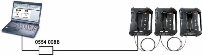
The individual components (e.g. Control Unit with meas. box or meas. box with meas. box) can be connected to a bus system using the Testo Data bus cable.
