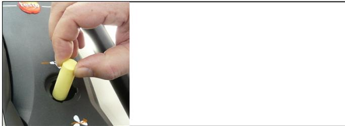
2. Remove the dirt filter and replace it with a new one 0554 3381).
