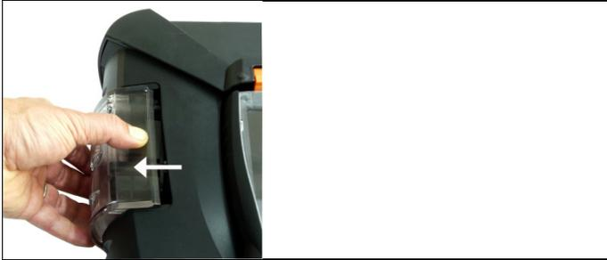
2. Unlock the condensate trap / condensate container and pull it vertically off the meas. box.
