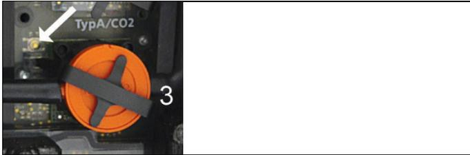
3. Hold the button at slot 3 carefully depressed with a pointed tool.
