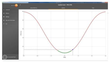
Via the first tab **Characteristics** and the field **Display properties**, you can change the clothing and activity parameters in the next window. This recalculates the PMV/PPD values and also the graphic. In order to be able to compare different calculations/graphics with each other, you need to save the respective CSV and PDF files. The calculations are overwritten in each case - it is therefore not possible to view different results of a measurement at the same time.
