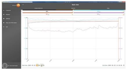
The total measurement period in the example in the figure above is 60 minutes. After changing the start time, only the last 10 minutes of the measurement are displayed in the graphic in accordance with the selection. Adjusting the time enables the measuring values to be analyzed in detail.
