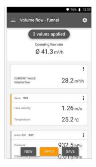
6 Apply: the current reading is applied.
