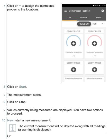
**Save**: exit the current measurement and save all readings on the testo 400 (see Section 9.6).
