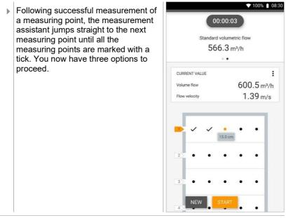
It is also possible to correct and overwrite individual measuring points by selecting the corresponding point on the display and starting a new measurement.
