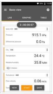
The counter in the upper section turns orange and measures the time (after stopping, the counter turns grey again). To the left of the counter, the number of the current/last measurement is displayed (e.g. 3 | 00:00:07 – the third measurement ran for 7 seconds).
