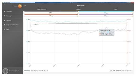
Clicking on one of the four channels opens the selection of measurement parameters recorded during the measurement. The measuring parameters can easily be assigned to the individual channels via the probe ID and measuring unit or selected as **not assigned**.
