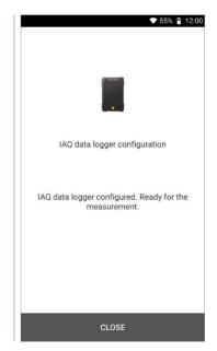
Following successful configuration, the testo 400 can be disconnected from the IAQ data logger. The measurement starts at the defined time or as soon as the setup has been completed (if the start time has been set to manual). The green LED on the IAQ data logger flashes rapidly at short intervals.
