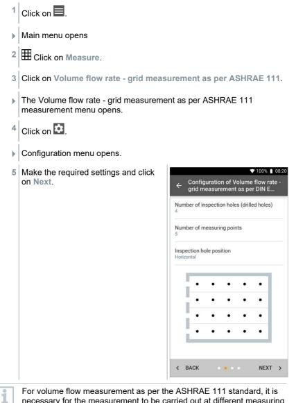
For volume flow measurement as per the ASHRAE 111 standard, it is necessary for the measurement to be carried out at different measuring points. The number of measuring points depends on the distance from the point of discontinuity and irregularities in the profile. In contrast to standard EN 12599, the measurement must be carried out on at least 5 inspection holes (drilled holes) and at 5 measuring points in each case.
