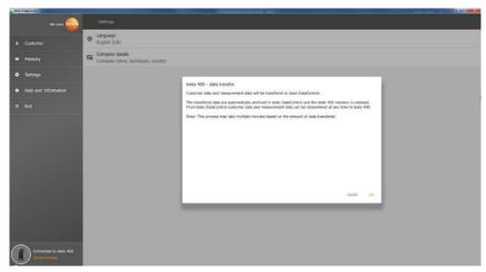
As soon as the testo 400 is connected via a USB cable to a computer, **Connected to testo 400 – Synchronizing** is displayed at bottom left. A message about data transfer is displayed. Confirm by pressing OK to transfer all customer and measurement data from the testo 400 to the software. The testo 400 memory is then empty. Depending on requirements, customer and measurement data as well as measuring site information can be transmitted back.
