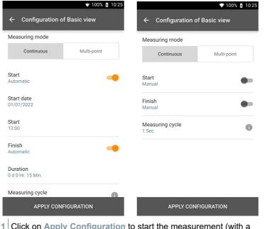
Click on Apply Configuration to start the measurement (with a scheduled start time).
