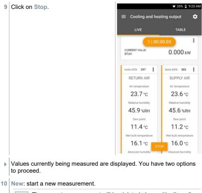
The current measurement will be deleted along with all readings (a warning is displayed).
