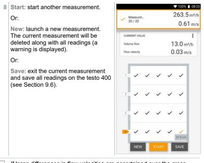
If large differences in flow velocities are ascertained over the crosssection, the number of measuring points must be increased. The number of measuring points is then adequate if the measurement value for each area is representative for its immediate surroundings, i.e. if it can be regarded as a genuine mean value for its portion of the area.
