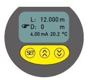
L=Level: from the bottom of storage to surface of the target
