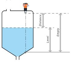
D=[C•T]/2 D: distance C: sound velocity T: time of flight
